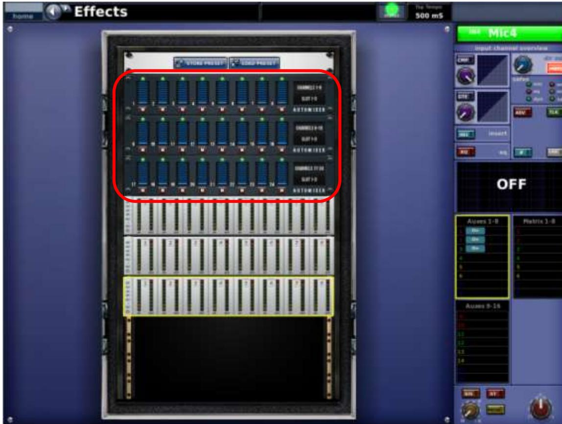
The Automixer can be cascaded. Up to 3 devices in the effect rack will act as one device.
