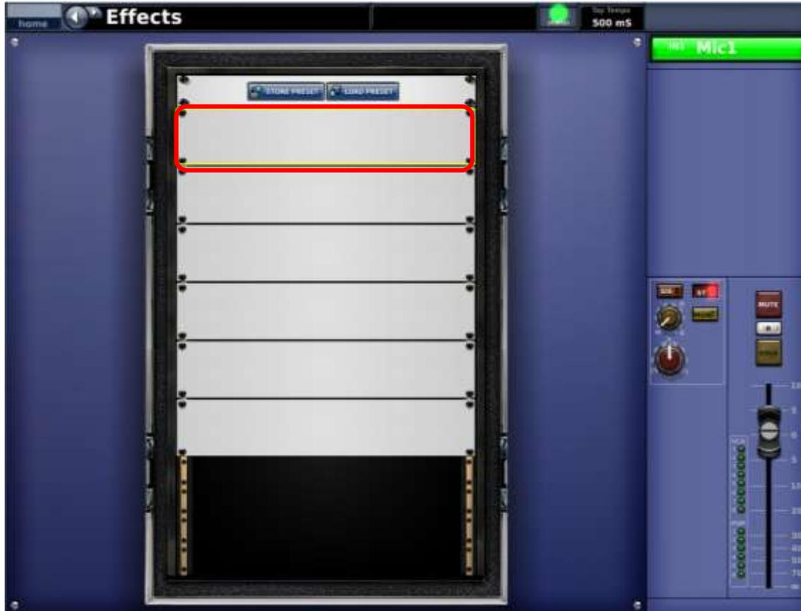
An 8-channel automixer can be installed in each of the available slots.
