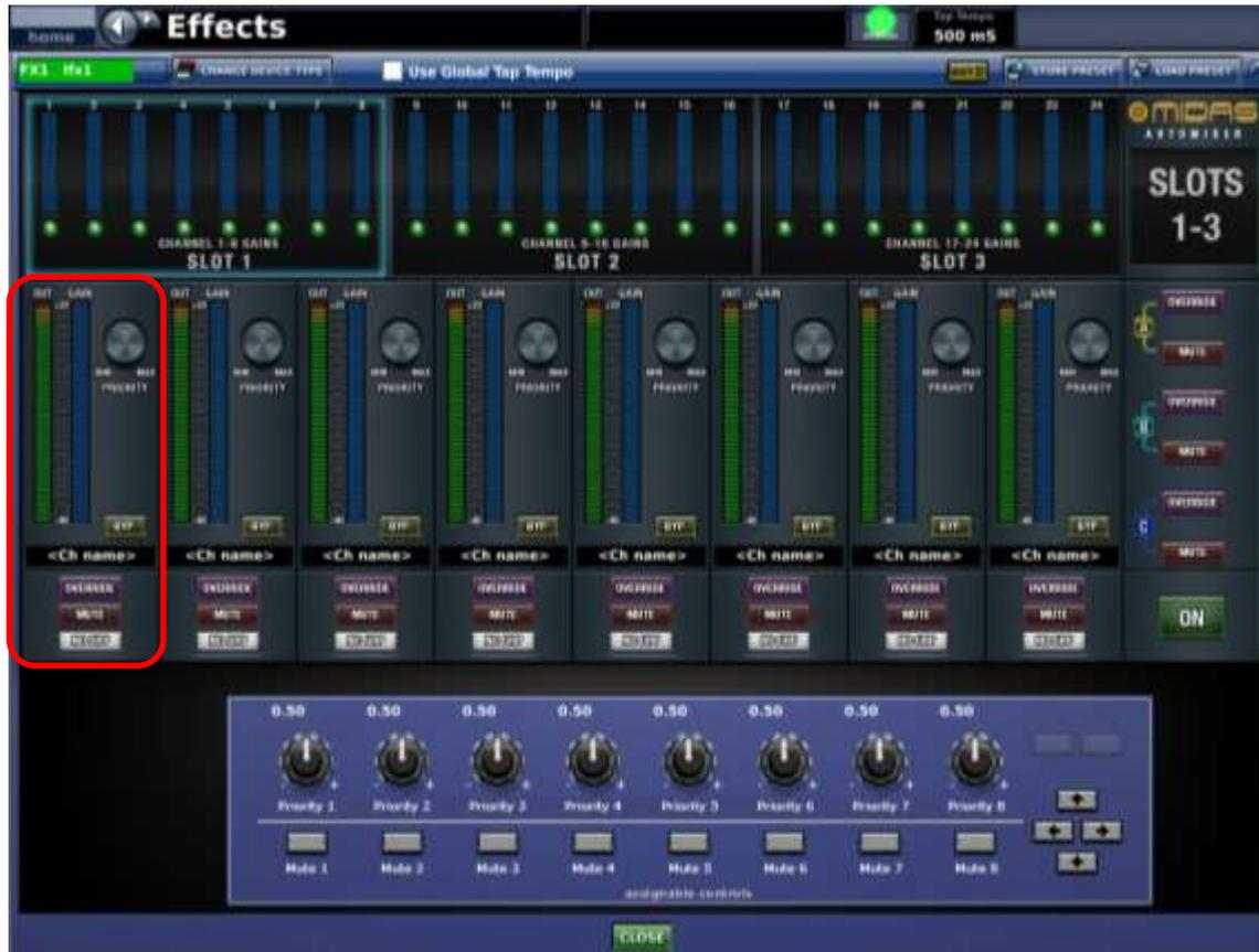
In each channel of the Automixer there are two meters: input signal and gain (blue meter). There is also an "OVERRIDE" button and a "NO GRP" button, which allows you to assign to any of the 3 groups.
