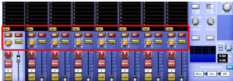
The best way to connect the Automixer is to use direct outputs. They should be set in such a way that the signal is picked up after the **fader** and **mute**. This can be done in the configuration section of each input channel. In this method, channels are not routed to main buses.
