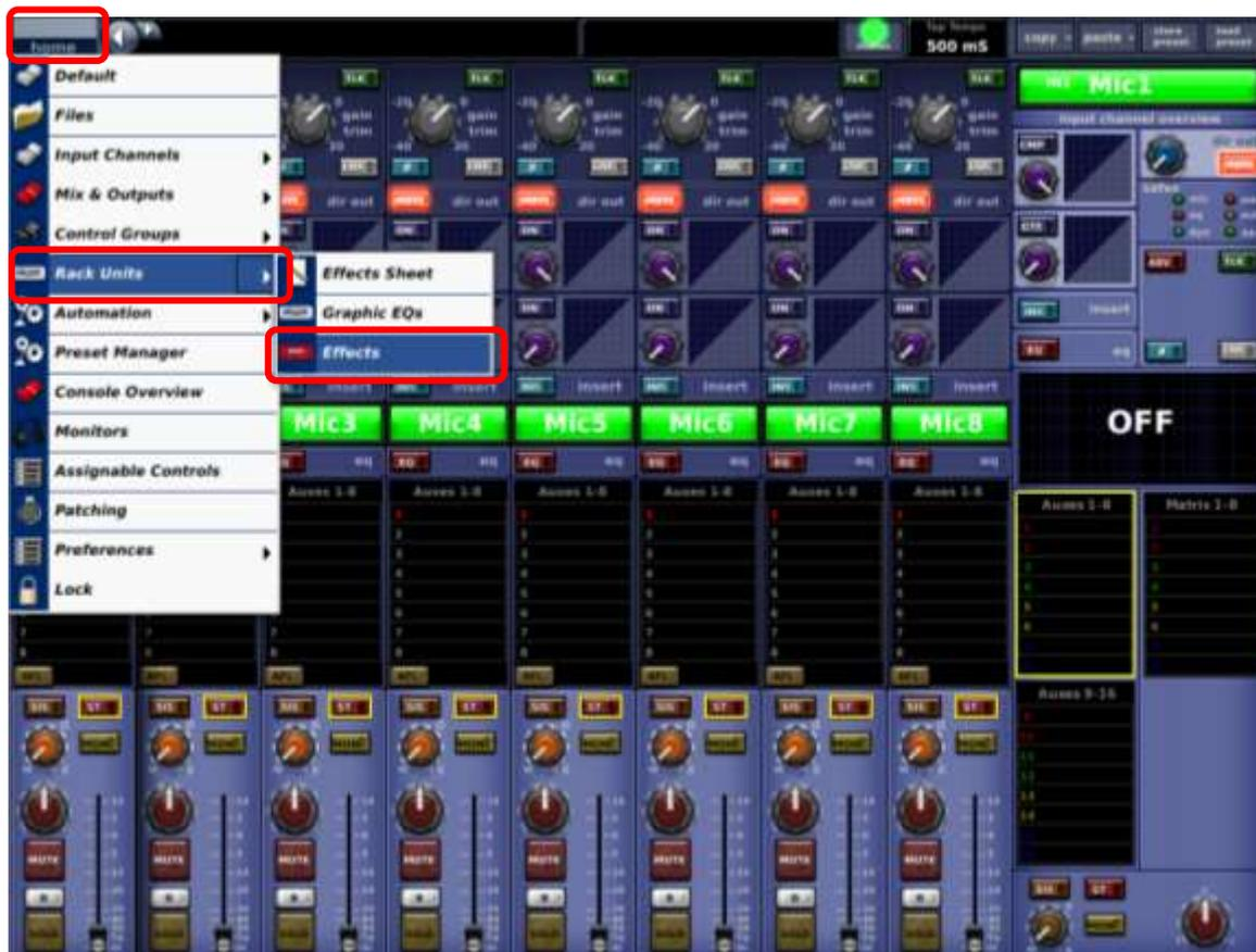
The first step is to “install” the automixer in the virtual effect rack of the console.
