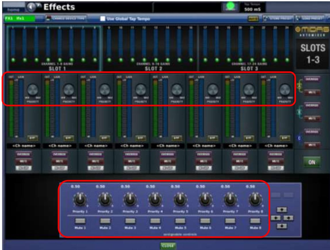
The device has 8 input channels and 1 output channel. The output channel of the Automixer should be patched to:
