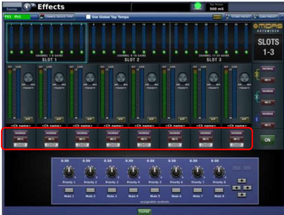
By default, the device acts as an 8-channel Automixer. This means that we can control 8 signals at the same time. Depending on the settings of the "PRIORITY" parameter, some may be varied in level more than others.
