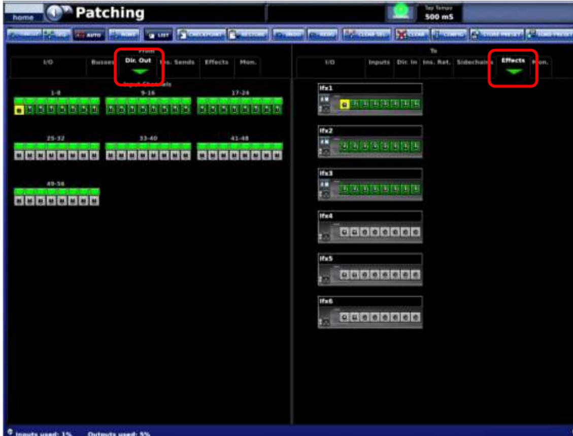
To send signals from channels, navigate to the patching screen and select DIR OUT and the EFFECTS tabs. Then select the channels you wish to use and connect them with the inputs of Automixer.
