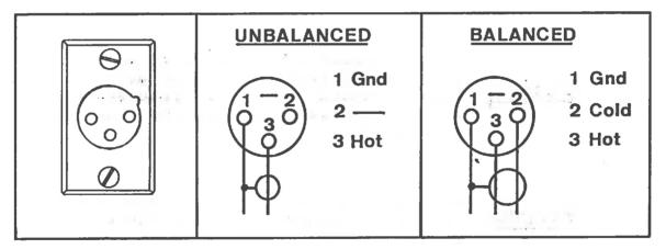
The input and output specifications make the DN27A readily compatible with the best professional quality equipment. One point regarding signal levels should however, be made. High level input signals should be attenuated sufficiently to allow gain in the equaliser section without exceeding the output clipping level. Transients should also be considered and adequate level headroom be allowed to process these accurately.
