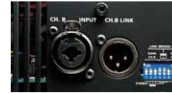
Neutrik Combo® input jacks adapt to both worlds, XLR or 1/4" phone plugs.
