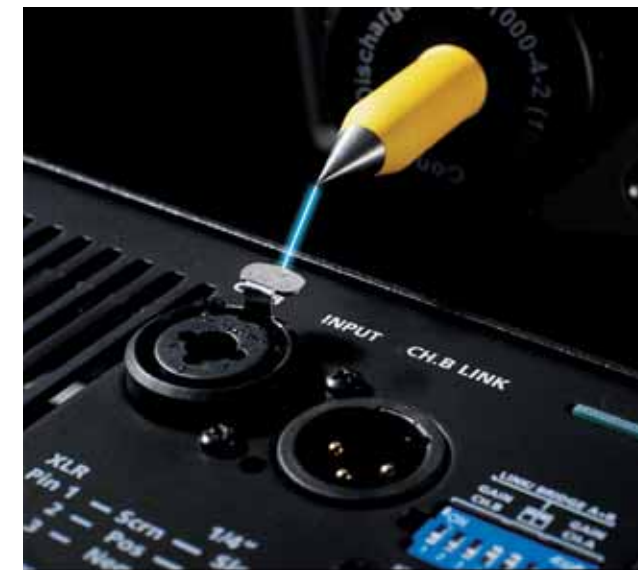
Lab.gruppen's EMC testfacilities. 8,000 volts are being "shot" with this gun for testing
