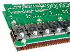
Output drivers are located side-by-side in the airstream.
