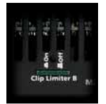
Recessed bypass switch per channel for the clip limiter.
