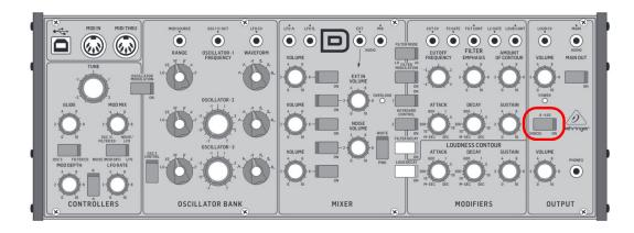
Switch the "A440" switch 4 times within the first 5 seconds after power up to disable the Poly Chain. You will see the power LED flash 4 times slowly to confirm Poly Chain has been disabled.
