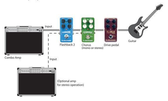
When using the Flashback 2 before the amp's input, it is generally best to place it after your other pedals. If any stereo effects are used before the reverb pedal, you can preserve this stereo signal by connecting to both of the Flashback 2's inputs and sending the output jacks to different amps or to a stereo input on a mixer.
