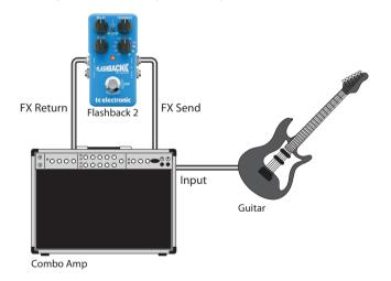
The Flashback 2 has a very wide gain range, and can easily be used with guitar or loop-level signals. Simply connect the amp's Send jack to the Flashback 2 input, and connect the output to the amp's Return jack.
