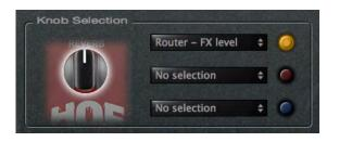
Knob Selection section of the TonePrint Editor for Hall of Fame Mini Reverb. This pedal has only one knob, which can still control up to three parameters.
