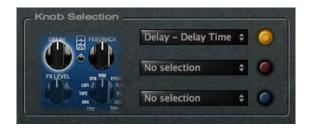
Knob Selection section of the TonePrint Editor for a Flashback Delay. Select a knob by clicking it, then select parameters from the three drop-down menus to define the parameters this knob should control.
