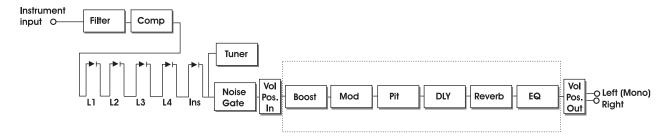
The Serial routing connects all Effect Blocks "in a straight line", similar to a regular guitar stomp box setup. This means that each Effect Blocks affects the following effect(s).
