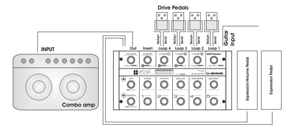
In this setup, we are using up to four drive pedals and a single combo amp. If you add another amp, you have a stereo setup.
