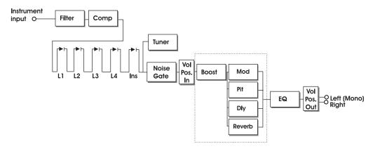
In the Parallel routing, the same signal is fed to the input of the Modulation, Pitch, Delay and Reverb sections, and therefore these effects will not affect each other.
