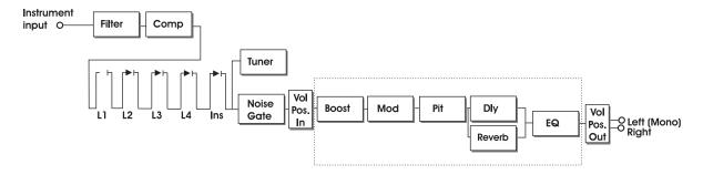
The Semi Parallel routing connects most Effect Blocks serially, but the Reverb and Delay blocks are now connected in parallel. Consequently, the Delay and Reverb effects do not affect each other. This means that e.g. the repeats of the Delay are not reverberated.
