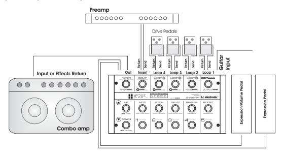
This setup is similar to the one described in the first example, but we have now added a pre-amp to the Insert loop. You can decide to have the pre-amp in or out of the signal chain per preset, but you will probably prefer to have it "on" at all times. This is configured in the Utility menu, which you can access in Menu Mode.
