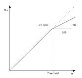
As this illustration shows, the output signal is attenuated in accordance to the set ratio when the input signal exceeds the Threshold point. The Attack parameter specifies how fast the attenuation is achieved. Use the Gain parameter to compensate the overall loss of level that might result from compression.
