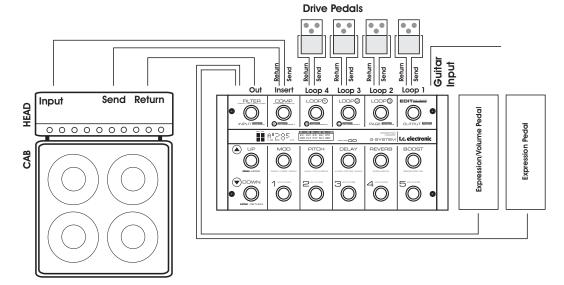
In this setup we are using a head as both pre-amp and power amp. The pre-amp section of the head is connected to the G-System's Insert loop. Set the Insert loop to "on" on all G-System presets, using the Utility menu.
