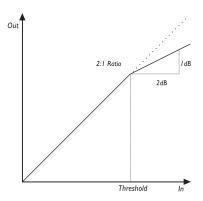
As this illustration shows, the output signal is attenuated relative to the set ratio when the input signal exceeds the threshold point. The attack parameter specifies how fast the attenuation is achieved. The Level parameter allows you to manually compensate for the perceived level difference resulting from compression.
