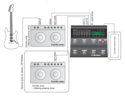
In this setup we use the preamp section of your combo amp to generate the drive. We use the Line input on the NOVA System and thereby bypass the NOVA Systems drive section. An expression pedal is connected to pedal in for real-time control of e.g. volume.
