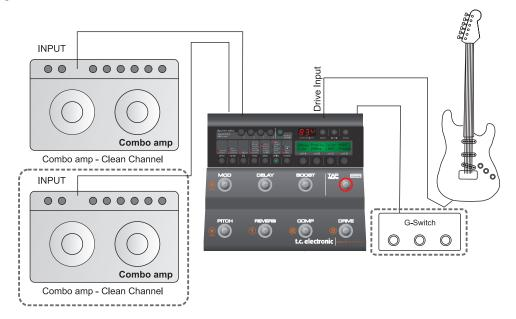
This is a typical basic setup combining NOVA System with one combo amp (or two for stereo) running a clean channel. All effects and overdrive/distortion are generated by NOVA System. A G-Switch (optional) is connected and the NOVA System is then automatically in stomp mode. Presets are then recalled using the G-Switch.
