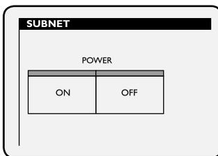
The Power OFF/ON buttons enable the user to switch the mains power state for ALL connected amplifiers in the local subnet. A green LED above each button indicates current status, either off or on. The power sequence delay time, dictating the time between power up activation of each consecutive amplifier in a subnet, can be adjusted.
