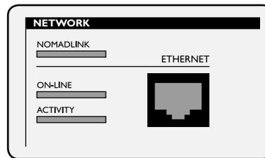
The front-panel Ethernet connection is located at the far right of the front-panel, adjacent to the network status indicators.
