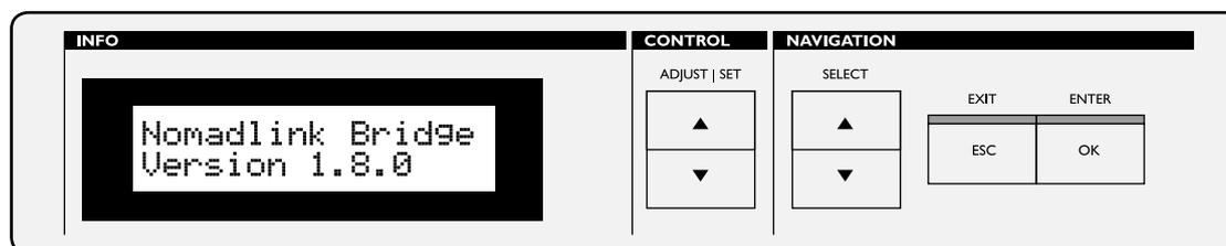
Use the six keys to the right of the 2x16 character LCD screen to navigate through the menu views of the NLB 60E. The views are organized as a tree-structure. Selecting "OK" when the display shows "Enter" will take you into a new set of selections. For an overview of all available displays, please refer to the Appendix section. In brief, to navigate the options you will:
