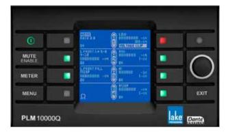
**The front panel** is the "local control center" for the PLM 10000Q. An intuitive, menu driven interface allows quick access to key functions using the moisture resistant silicone touchpad. Information is clearly displayed on the daylight-readable, 2.5-inch LCD panel. The soft-button keypad and precision rotary encoder provide control of processing and amplification functions, with key lock available.
