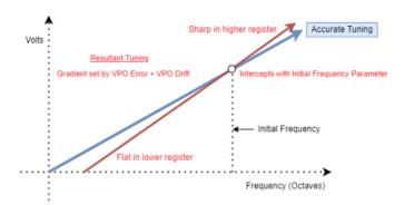
The above graph applies to FVPO Error, FVPO Drift, FDrift Speed and FInitFreq in relation to the filter where frequency is in relation to the frequency of the resonant peak of the filter; OSCVPO Error, OSCVPO Drift, ODrift Speed and OSCInitFreq where frequency is in relation to the pitch of the oscillators. These parameters allow the tuning of the filter to be adjusted emulating volts per octave calibration tuning error in vintage synthesizers.
