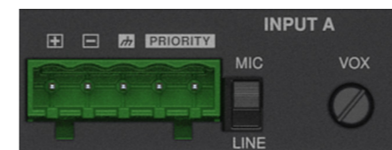
5-Pin Euroblock Connector - Remote
