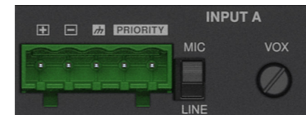
5-Pin Euroblock Connector - Remote
