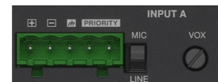
5-Pin Euroblock Connector - Remote
