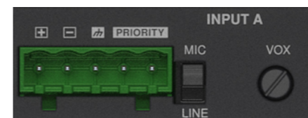
5-Pin Euroblock Connector - Remote
