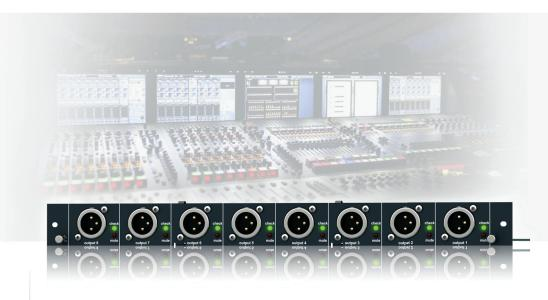
DL442 is a modular 8 analogue line level output card for MIDAS PRO Series control centres and modular I/O boxes, and features servobalanced electronic outputs with high output current drive capability for long cable runs. Premium low latency 24 bit 96 kHz DAC converters are used to minimise distortion and noise artefacts and DL442 features an automatic output mute facility if the
