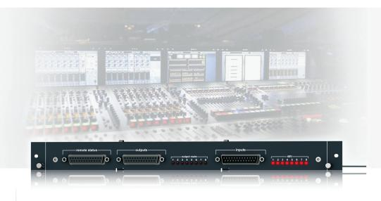
DL444 is a modular 8 channel analogue mic/line input and line level output card for MIDAS PRO Series control centres and modular I/O boxes, and features award-winning MIDAS microphone preamplifiers with switchable +48 V phantom power and servo-balanced electronic outputs with high current drive capability for long cable runs. Premium low latency 24 bit 96 kHz ADC and DAC converters
