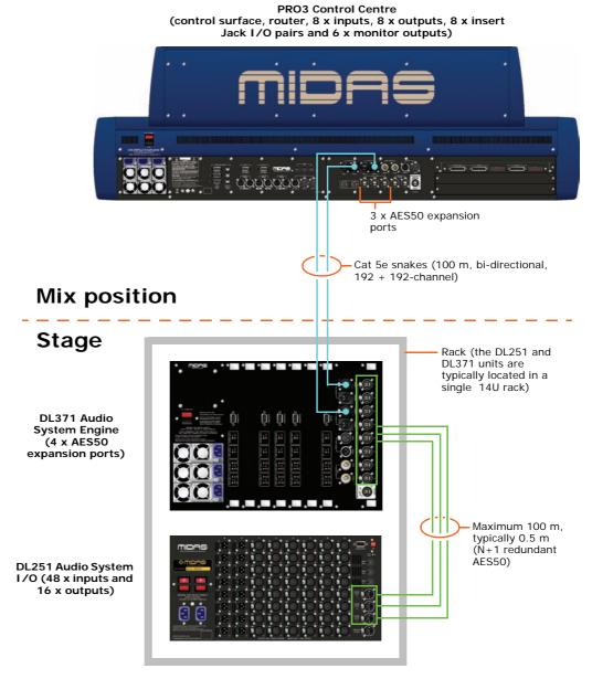
Figure 7: Standard PRO3 system configuration
