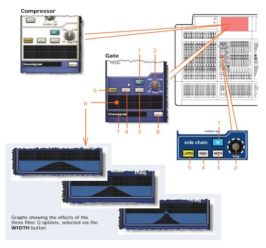
Side chain controls for the input channels on the control surface and GUI
