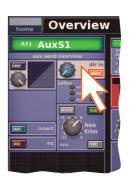
Click MODE repeatedly to scroll through the mix modes (mix, group and mix minus) to select the one you want. Group mode is fader only with no pre-fader, and in mix minus mode all buses are initially routed — you have to turn a bus routing switch on to take it out of the mix. Stereo mix mode — with mix selected and LINK button on — is only accessed from the odd numbered output channel of the linked pair. In stereo mix mode the top control knob becomes pan adjust and the bottom one adjusts level.
