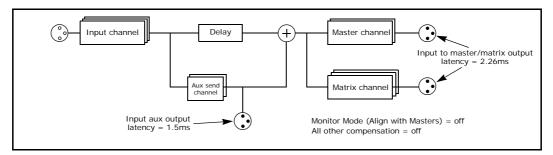
Figure 28: Routing via the aux send buses
