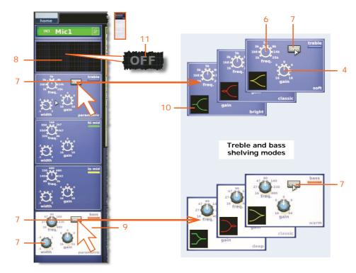
EQ controls for the input channels in the GUI channel strip. Shows the treble and bass modes, selected via the **SHAPE** buttons.
