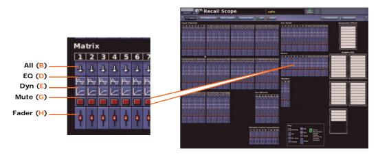
Parameter sections per matrix channel. There are 16 matrices per PRO6 and PRO9, and only eight on the PRO3. This example is taken from a PRO9.
