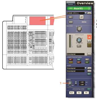
Insert and configuration processing area in GUI channel strip
