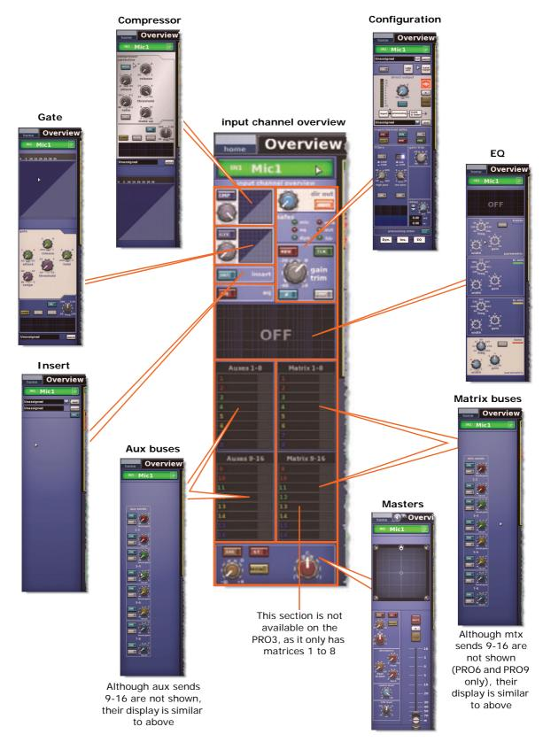
Figure 34: Processing areas available from the input channel overview display
