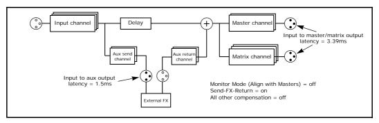
Figure 27: Routing via the aux send and return buses
