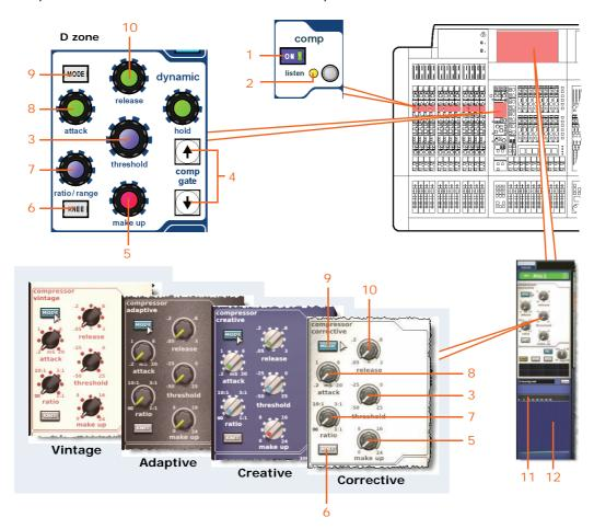
Compressor types and their input channel controls (control surface and GUI)
