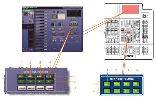
Talk osc/routing controls on the control surface and GUI
