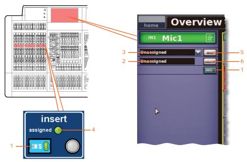
Insert controls for the input channels on the control surface and GUI
