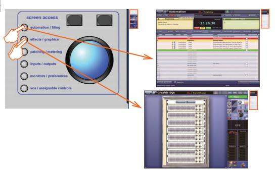
These two examples show you how to use the **screen access** buttons to open the **Automation** screen (single press) and the **Graphic EQs** screen (two presses). These buttons take you directly to the screen you want.
