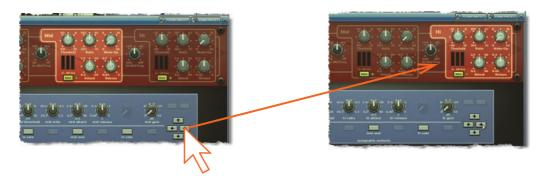
In view 2/4 of the 3-band compressor effect the I zone is assigned to the **Mid** section. Clicking the right arrow takes you to view 3/4, and the I zone is now assigned to the **Hi** section. If you clicked the left arrow instead, this would take you in the opposite direction to view 1/4, and the I zone would be assigned to the **Lo** section.
