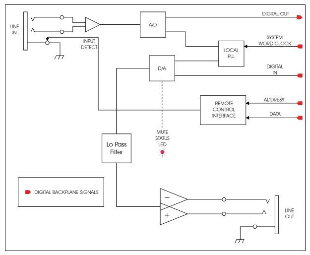
Functional block diagram of the DL443 module
