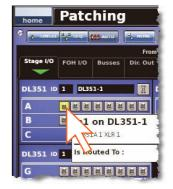
3 Select the destination patch connector. For example, in the **Inputs** tab of the **To** section, click the patch connector for input channel 14 (Mic14). It will now be patched to the source. If the new patch is carrying a signal, this audio may be heard, depending on the settings of the control centre.
