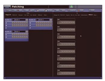
Patching screen showing the location of the effects in the Effects tab of the To section. (PRO3 only has a maximum of six effects.)
