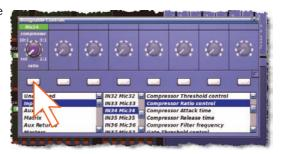
An alternative method is to press and hold down an I zone assign/unassign button in the assignable controls of the control surface. Then, on the GUI (maser bay screen), click the desired control.
