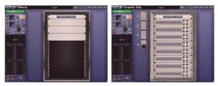
Typical **Effects** and **Graphic EQs** screens as configured for the **3 Effects - 28 GEQs** option. Note the four small racks to the left of the main rack on the **Graphic EQs** screen, which cater for the 28 GEQs; the selected rack unit is highlighted in yellow.
