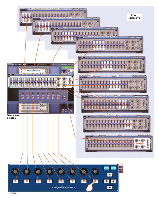
Figure 24: I zone LCD button assignments in the overview display
