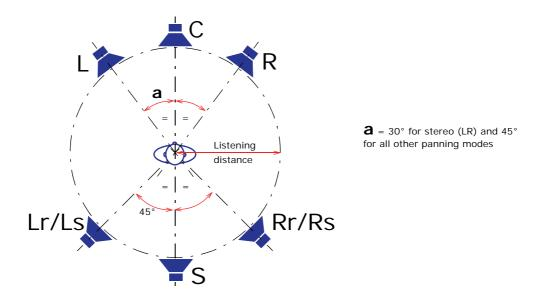
Typical examples of loudspeaker placements for each panning mode (see Table 7 "Panning formats" on page 131). Please note that these are only an approximation and should only be used as a guide.
