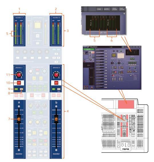
Figure 20: Monitor A and B strips
