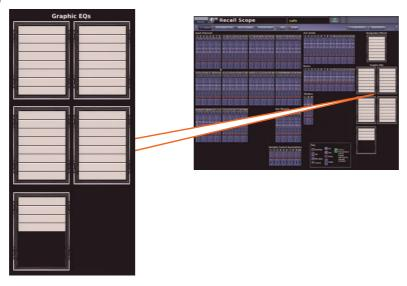
Graphic EQs represented on the **Recall Scope** screen. Racks are always shown fully populated, regardless of how many GEQs are configured. This example is taken from a PRO9.
