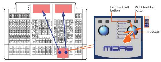
Figure 9: Controlling the GUI
