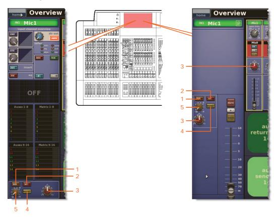
Input channel masters controls on the GUI
