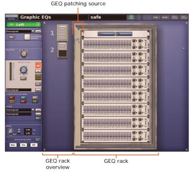
Figure 21: Graphic EQs screen (configured for 12 GEQs)
