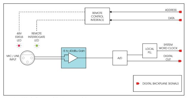
Functional block diagram of the DL441 module
