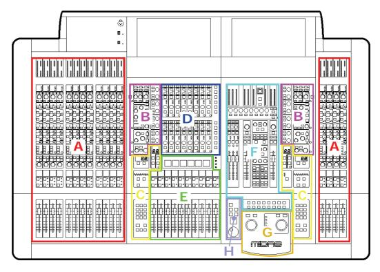
A — input fast zone: 16 input fast strips across the 12-channel and 4-channel input bays provide the operator's 'must have now' controls.
