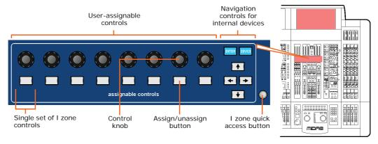
Figure 22: I zone controls on the control surface
