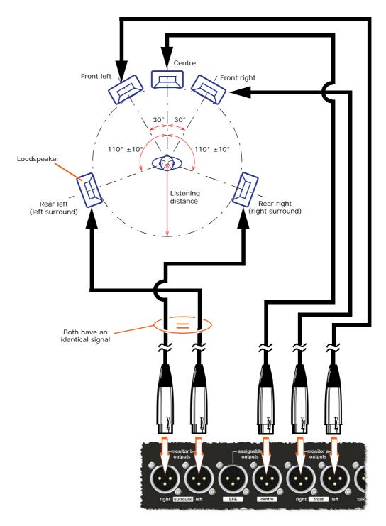
Figure 32: Connections for an LCRS surround system (with recommended speaker set-up)
