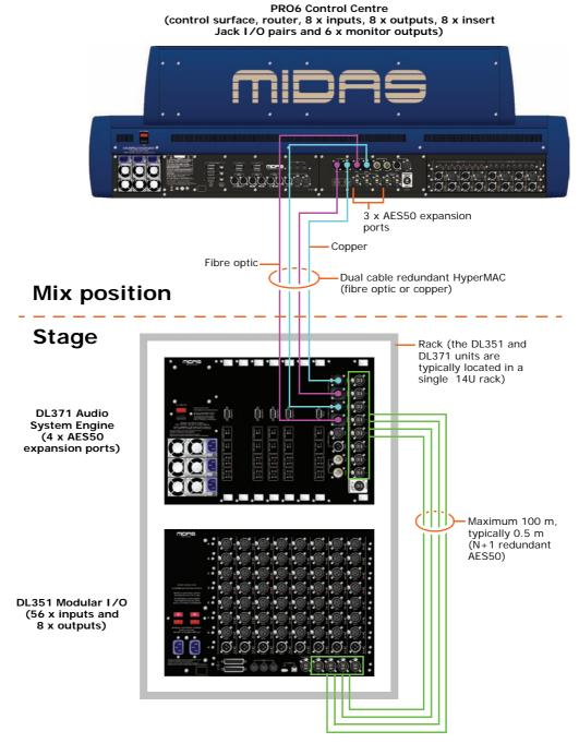
Figure 8: Standard PRO6 system configuration
