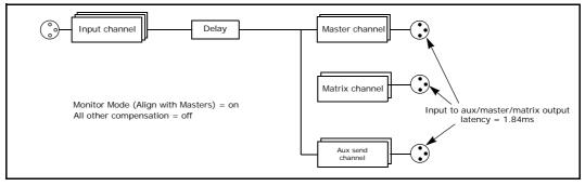
Figure 29: Latency for normal routing
