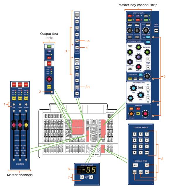
Figure 12: Output channel navigational controls
