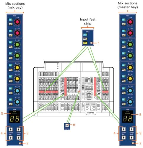
Figure 11: Mix bus navigational controls
