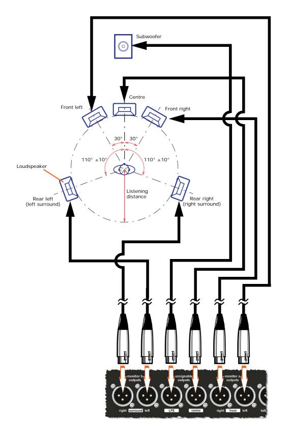
Figure 33: Connections for a 5.1 surround system (with recommended speaker set-up)
