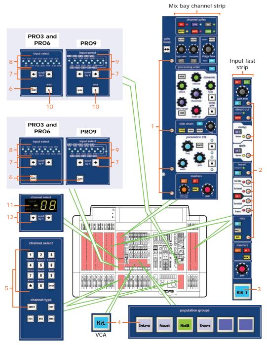
Figure 10: Input channel navigational controls
