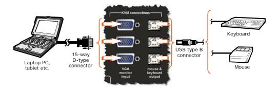
KVM connections on the rear panel of a PRO Series Control Centre
