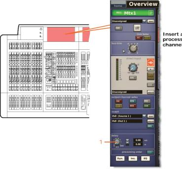
Insert and configuration processing area in GUI channel strip
