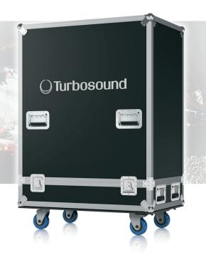
The TLX84-RC4 road case, for up to 4 TLX84 line array elements, is designed to withstand the rigours of live concert touring. It is constructed from 12 mm rigid plywood with 40 x 40 mm durable aluminium edging extrusions. High density foam provides internal support and superior protection in transit, night after night, city after city.
