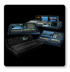
MIDAS PRO and M32 Series digital consoles, enabling a digital snake connection from Front of House to stage.
