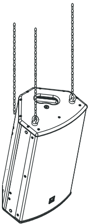
Suspension using M10 shoulder eyebolts
