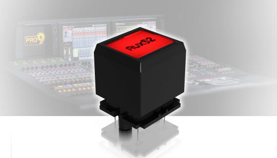
PRO LCD SWITCH enables dynamic and context-sensitive user interfaces, providing clear visual feedback of assigned functions and user-created labelling of mixing console channel, bus and group selections. The high contrast FSTN LCD glass with 36 x 24 pixel resolution allows immediate at-a-glance indication over a very wide viewing angle, and the tactile response of the momentary switch
