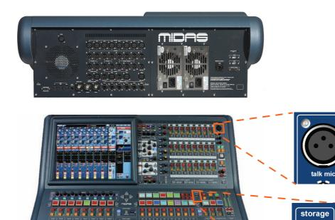
Rear panel connectors (top) and storage USB connector on the control surface
