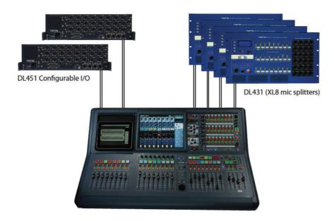
PRO2 system expanded by adding DL431 input splitters and DL451 modular I/O boxes
