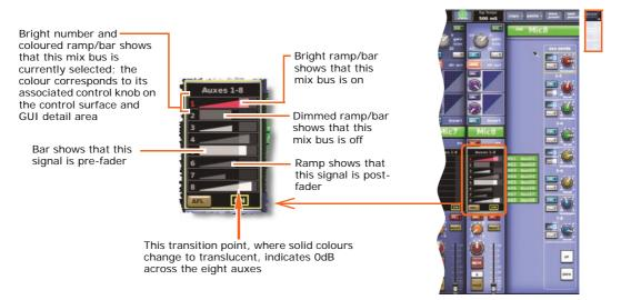
Figure 7: Typical mix section in a GUI input fast strip
