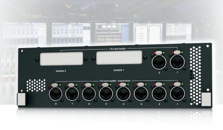
The NEUTRON-NB Network Bridge expansion module compatible with the MIDAS NEUTRON audio system engine provides a multichannel interface between two third party digital audio networks and point-to-point interfaces. The third party interfaces operate in separate clock domains and are connected by a bidirectional asynchronous sample rate converter (ASRC). This unique
