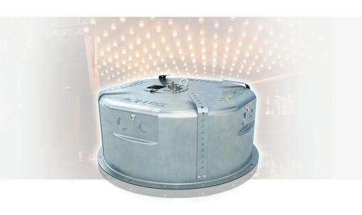
The CMS 801 PI 8 OHM BACKCAN is an acoustically enhanced zinc plated steel back can designed for the pre-installation of CMS 801 PI loudspeakers in newly constructed, non-suspended ceilings. Early installation of the low profile back can is fast and simple via the included flexible metal straps, and significantly reduces the amount of time required for project
