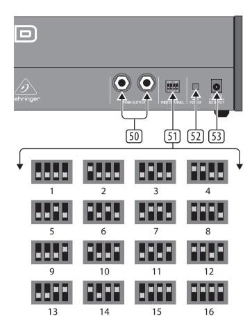
MAIN OUTPUT - connect these 1/4" TRS outputs to the inputs of your external equipment as follows (note that they are both Mono, and not left/right):
