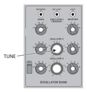
8. Turn the front panel OSC2 Octave RANGE knob to the 8' position.
