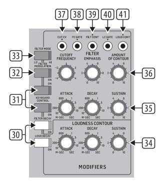
DECAY - when ON, the signal will decay during the time set by the DECAY TIME knob after a note or external trigger is released. When OFF, it will decay immediately after a note or external trigger is released.
