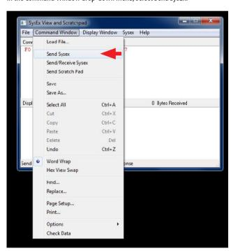
The SysEx message will be sent to the MODEL D, and it will then be in its PITCH Calibration mode. 8. If you wanted, you can use the SAVE AS command in the Command Window drop down menu to save the SysEx message as a file on your computer for later use.
