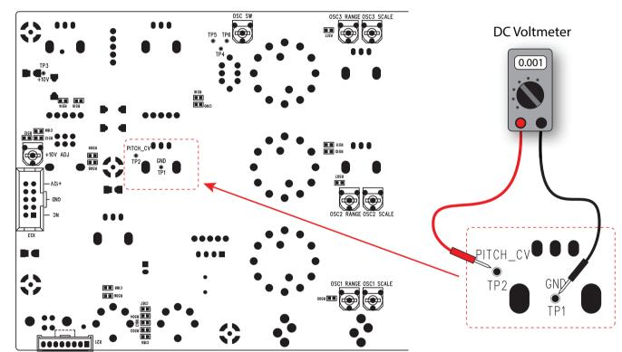
7. The keyboard diagram on the next page shows the keys used during the PITCH CV calibration procedure. The calibration requires setting three values: Low, Zero, and High. Various keys on the external keyboard are used to select and trigger these three different calibrations, to adjust the voltage readings, and to Save and Exit the procedure..
