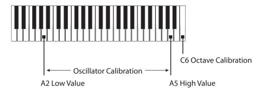
10. Listen carefully, and adjust the OSC SW trimpot on the PCB, for zero beats between OSC1 (Range=2') and OSC2 (Range=8').
