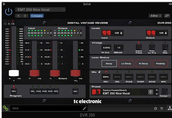
The plug-in is divided into two sections, which are both visible when the “I+II” button at the top left is selected. The left section is identical to the hardware unit and could be considered Primary parameters. These include common items such as delay time and feedback.
