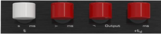
The levers often control certain types of parameters regardless of which effect is selected. For example, the 4th lever always controls the predelay as long as the primary set is active (SET button off). The first lever tends to control the primary time parameter for each effect.
