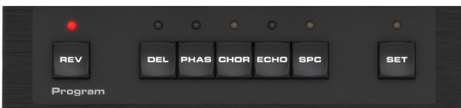
Activate an effect with the program buttons. The currently-selected effect will be indicated by a lit LED. Only one effect can be activated at a time.
