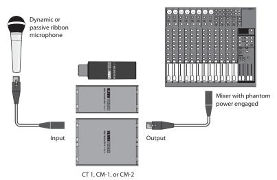
\*note – the CT 1 can also be connected directly to most microphones
