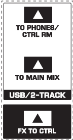
Fig. 2.12: Assignment switches of the main section
