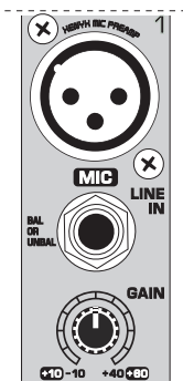
Fig. 2.1: Connectors and controls of mic/line inputs
