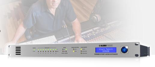
The DN9680 provides a high channel count solution to the 100 metre limitation that Ethernet and CAT5 cabling imposes on the physical size of AES50 networks. A pair of DN9680 units allow up to eight AES50 connections (192 bidirectional channels) to be extended by up to 1,000 metres via single mode optical fibre or 100 metres via CAT5 copper cable, greatly simplifying long haul
