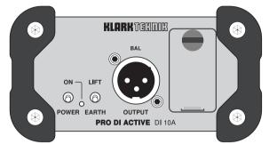
LIFT / EARTH – switch can be used to connect or disconnect the ground link between the INPUT and OUTPUT jacks in order to reduce hum or prevent group loops. The LIFT / EARTH switch's ability to reduce hum or prevent ground loops depends on the grounding of connected devices. When the switch is in the LIFT position, the ground connection between INPUT and OUTPUT is disconnected.
