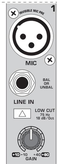
Fig. 2.1: Connectors and controls of mic/line inputs
