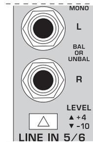
Fig. 2.5: Stereo channel inputs and LEVEL switch
