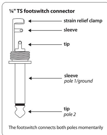
Fig. 4.1: 1/4" TS connector for foot switch
