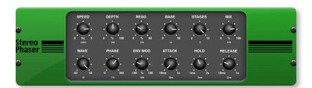
A STEREO PHASER, or phase shifter, applies multiple stages of modulated filters to the input signal to create a "notch" in the frequency response, and then blends it with the original for a "swirling" effect. Use the STEREO PHASER to add a "spaced-out" sound to vocal or instrument tracks.
