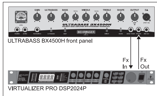
Fig. 3.4: Connection of a multi-effects processor
