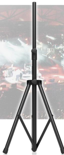
Designed to support mid-high loudspeakers fitted with 1 3/8" (35 mm) pole sockets in free-standing applications, the TSTAND-01 provides reliable and safe mounting with an adjustable height ranging from 4' 5" to 7' (1.35 m to 2.15 m). The steel tripod stand with a hard wearing semi matt black finish features a friction screw for easy and stable height adjustment, and an integral locking pin for added security.
