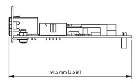
Audinate Dante Network Module with up to 64 Bidirectional Channels
