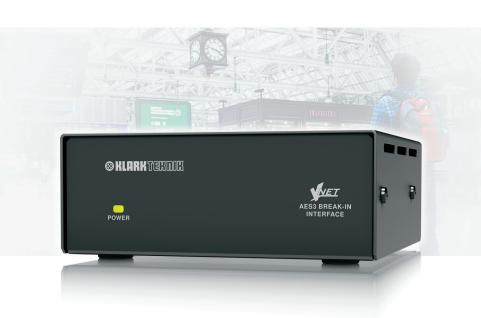
The VNET2-AES is a rack-mountable break in interface for connecting an AES3 source to the VNET network with the minimum of complication. The interface allows the facility of transporting 2 channels (one AES3 stream) of high quality uncompressed digital audio on the same cable as the control network. Capable of driving up to a 600 m (1,968 feet) network, VNET2-AES interface should be used
