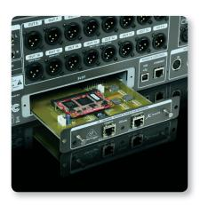
The X32's expansion slot provides flexible and expandable connectivity for many different applications. The X-DANTE Expansion Card can easily be installed in place of the X-USB card that is included with the X32. The 32-channel 48 kHz bi-directional audio interface brings even more I/O options to the X32 by making it ready for integration with Dante enabled IP networks.
